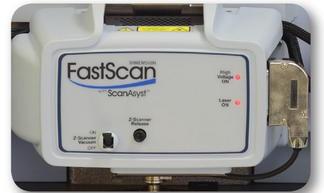
Scanner Resonant Frequency X-Y: 2.70kHz, Z: >50kHz.
